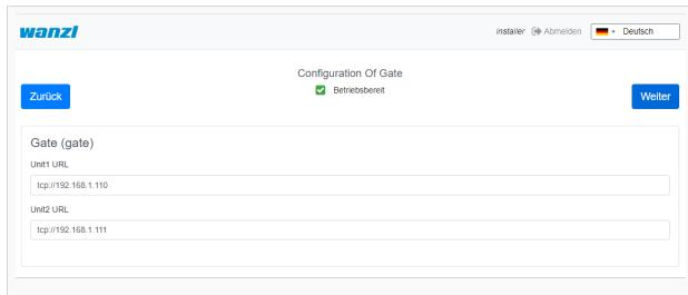
The screenshot shows a configuration interface for a 'Gate (gate)'. At the top, there's a header with the title 'Configuration Of Gate', a 'Zurück' button, and a 'Weiter' button. Below the header, there's a checkbox labeled 'Betriebsbereit' which is checked. The main area contains two input fields: 'Unit1 URL' with the value 'tcp://192.168.1.110' and 'Unit2 URL' with the value 'tcp://192.168.1.111'. The entire interface is in German, indicated by the language selection at the top right.
