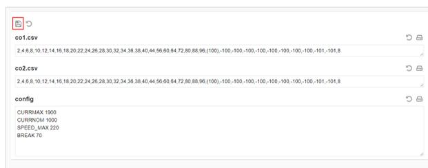
The screenshot shows a configuration interface with three sections: 'cof1.csv', 'co2.csv', and 'config'. Each section has a diskette icon for saving. The 'config' section contains the following parameters: CURRMAX 1000, CURRNOM 1000, SPEED\_MAX 220, and BREAK 70.
